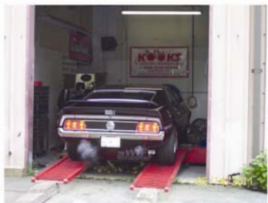
Dan Breton's 1971 Mach I was the first test subject. The Mach pulled 217 hp to the wheels
